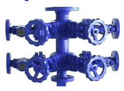
The compact condensate manifold with internal immersion tube and integral bellows-sealed globe valves and laterally arranged RHOMUBS *line* steam traps type MK 45 / BK 45.
